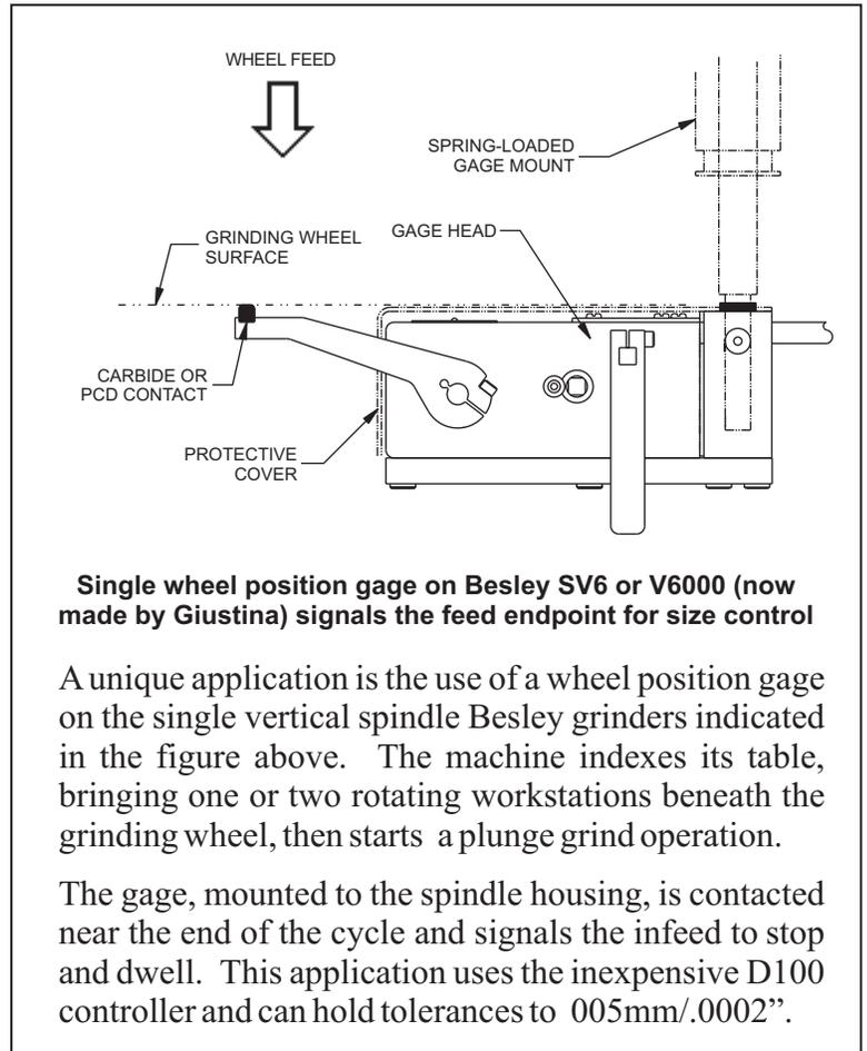
**Single wheel position gage on Besley SV6 or V6000 (now made by Giustina) signals the feed endpoint for size control**
